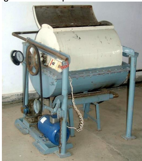
A field convenient jacketed leaf inactivator for green tea processing
