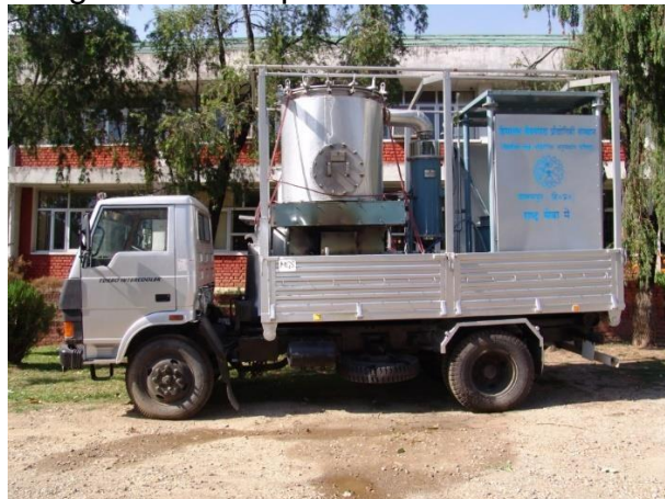
Mobile essential oil distillation unit
